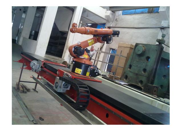
Linear Tracks are used in Robotic system as a 7<sup>th</sup> Axis movement for Robots. These tracks are specially made for Robot that can synchronous with robot movements and control by robot program.
